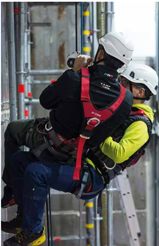
Two-person emergency descent test with a prototype of the Giant descender. Prueba de descenso de emergencia de dos personas con un prototipo del descensor Giant. Corde-Access SA training centre, Puidoux, Vaud, Switzerland (ph. Mauro Galimberti).
