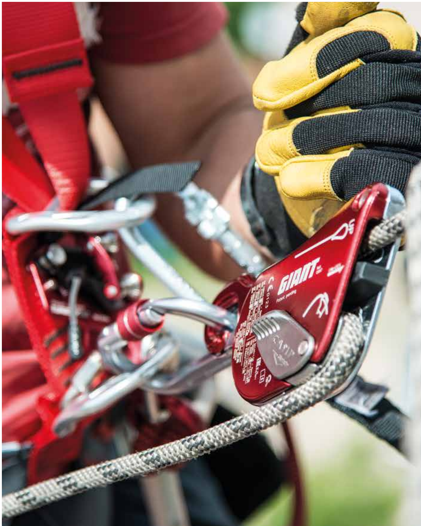
The Giant descender on the cupola of the Aquapark Nymphaea. Bajada con el descensor Giant encima de la cúpula del Aquapark Nymphaea. Oradea, Romania (courtesy of Camp Technical Solutions, ph. Riky Felderer).
